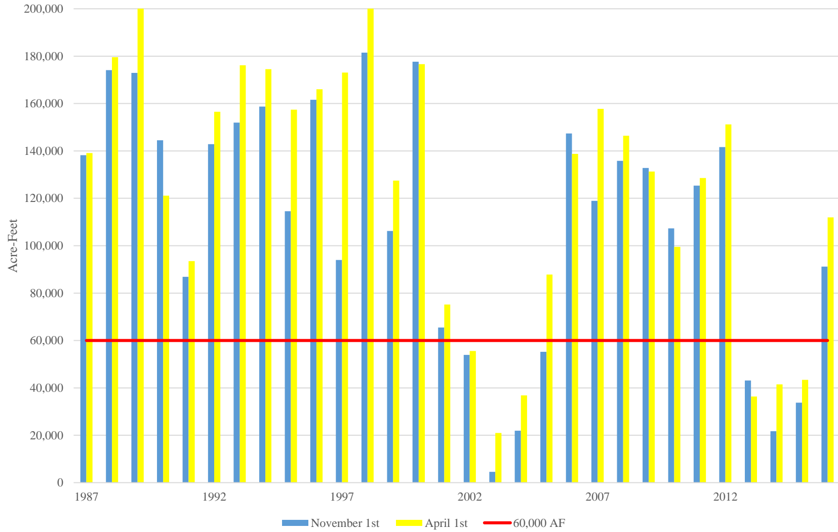
Figure 17. November 1 st vs. April 1 st McPhee Active Capacity
